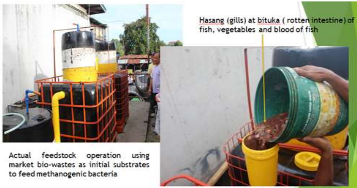
The actual operation of Twin IBC Water Tank Biogas Digester using fish gills, rotten intestine, and vegetables and blood of fish as a substrates.
